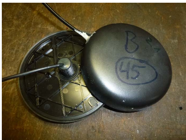
19. UUT after IP 6X, no penetration of dust visible
