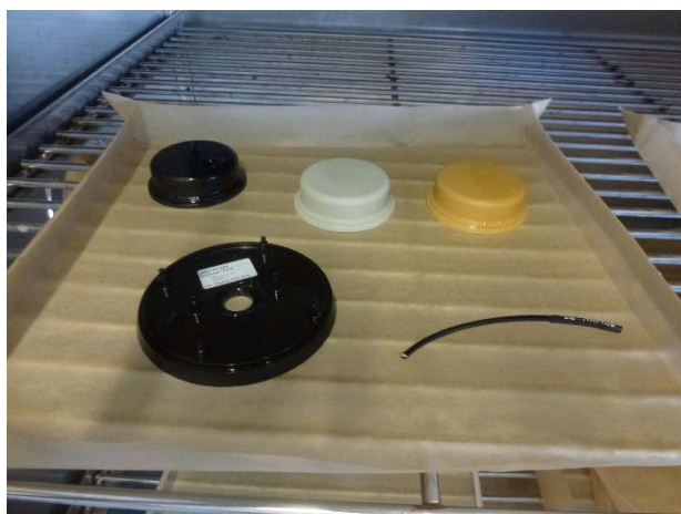
27. UUT during chemical resistance test in the climatic chamber
