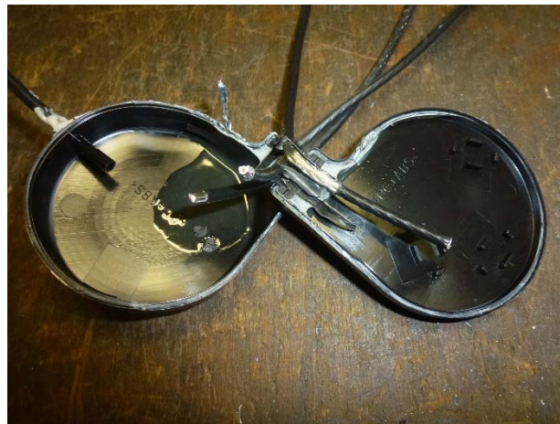
18. UUT after IP 6X, no penetration of dust visible
