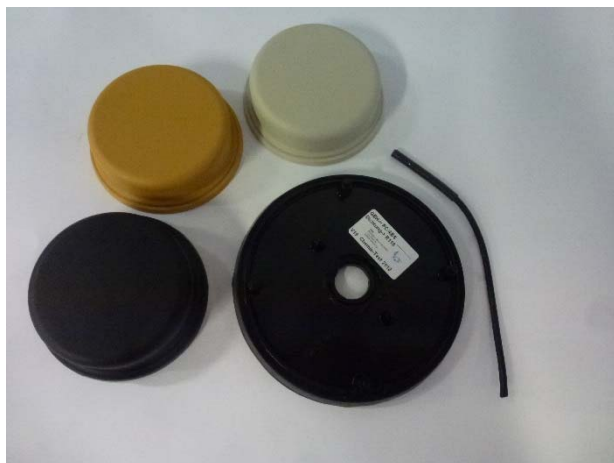
33. Chemical resistance test, UUT cleaned after chemical resistance test, no change visible
