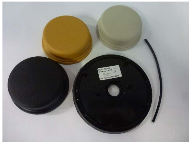
30. Chemical resistance test, UUT after 22 h at 85°C I the climatic chamber
