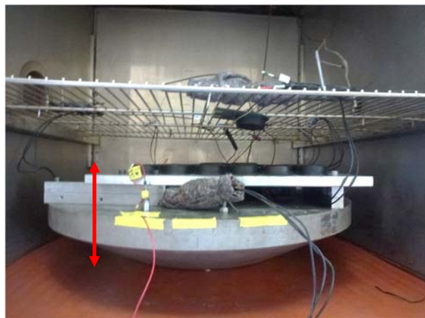
4. UUT during vibration with temperature overlay on head-expander in climatic chamber in Z-axis
