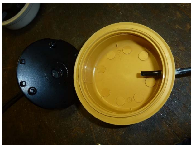
20. UUT after IP 6X, no penetration of dust visible
