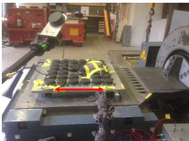
7. UUT during shock tests on slip-table in X- and Y-axis
