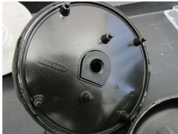
26. No penetration of water visible
