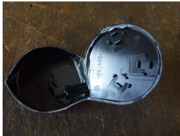
22. UUT after IP X7, no penetration of water visible
