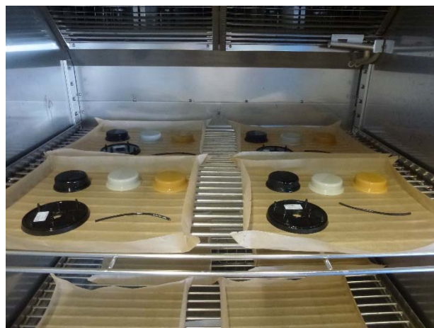
28. UUT during chemical resistance test in the climatic chamber
