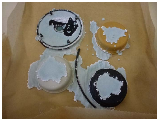
32. Chemical resistance test, UUT after 22 h at room temperature
