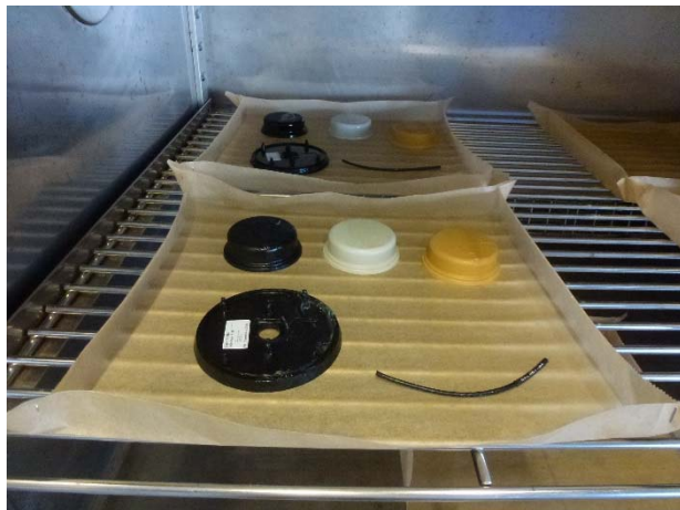
29. Chemical resistance test, UUT after 22 h at 85°C I the climatic chamber
