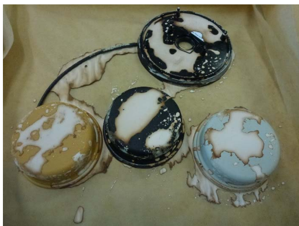
31. Chemical resistance test, UUT after 22 h at room temperature
