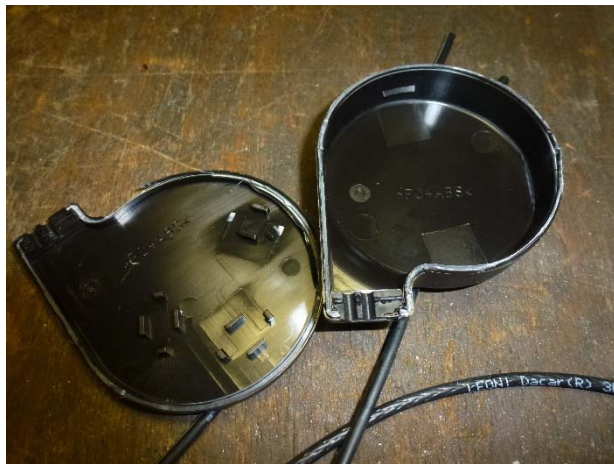
13. UUT after IP 54, no penetration of dust or water visible
