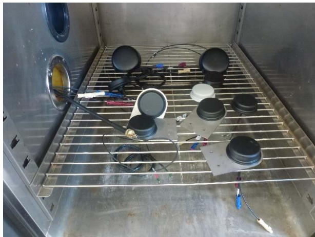
1. UUT in the climatic chamber
